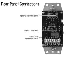
Input-Cable Connection Block — Using standard IDC punchdown tools, connect the Category 5/5e cable linking the AB 2 to the receiver or hub to this connection block in accordance with the color code printed on the circuit board.
